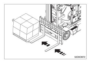
While traveling the forklift with the load on the side shift, if the operator lift or lower the load without shifting it in the netural position, it can be overturned the forklift due to unstabled load.
