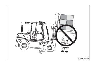
Never use wire rope to lift a load.
